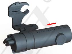
1 - To install the dashcam into the mount, simply squeeze the two tabs of the spring clip together as shown above. This will increase the diameter of the spring clip and allow you to slide the dashcam into position. Once the dashcam is in position, release the two tabs. The dashcam is now securely attached to the mount.
